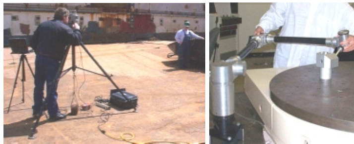
Manual measurement systems include the Total Station (left) and the Coordinate Measurement Machine (right)
