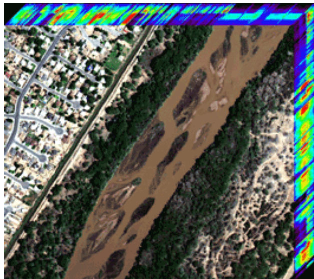
Hyperspectral imagery data cube enables automated classification of features, including delineation of land water interface, vegetation associations and dominant vegetation.
